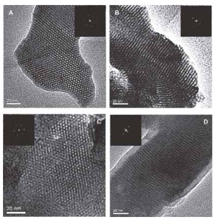
**Fig. 2.** TEM and (insets) FFT images. (**A** and **B**) As-prepared MSU-Ge-2. (**C** and **D**) Mesoporous MSU-Ge-2 obtained by heat-treating the NH<sub>4</sub><sup>+</sup>-exchanged material. The images shows a periodic hexagonal array along the [100] direction (A and C) and a periodic array of parallel pore channels along the [110] direction (B and D).
